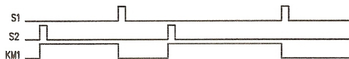
Figure 2. Graphic representation of the logic equation for direct start of the induction machine
