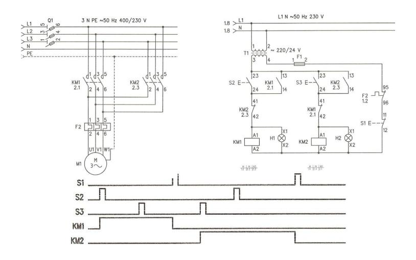
KM1 = (NOT KM2) AND ((S2 AND (NOT S1)) OR (KM1 AND (NOT S1)))KM2 = (NOT KM1) AND ((S3 AND (NOT S1)) OR (KM2 AND (NOT S1)))
