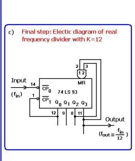
• programmable frequency dividers implemented with synchronous counters
